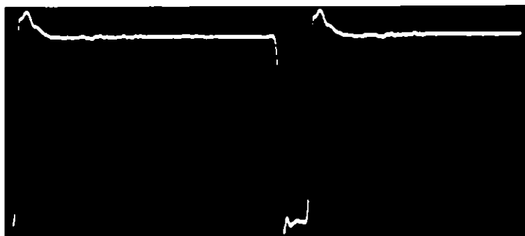
(a) Sweep speed set to 0.1 \mu\text{s}/\text{div} and no X expansion
