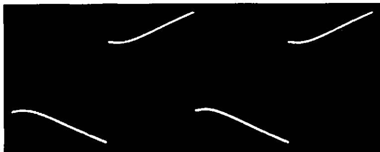
(d) Output with increased bass response, 1 kHz input
