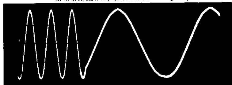
(c) Delayed triggered sweep method. Timebase B trigger set to positive slope and trigger control to 'low level'
