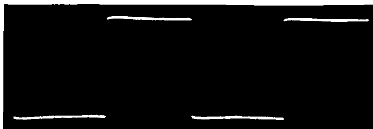
(a) Output with tone controls in central position, 1 kHz input
