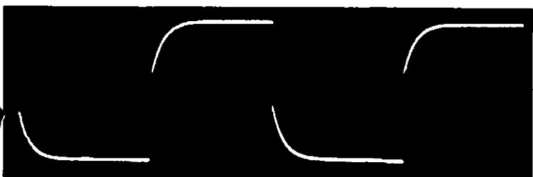
(c) Output with decreased top response, 1 kHz input
