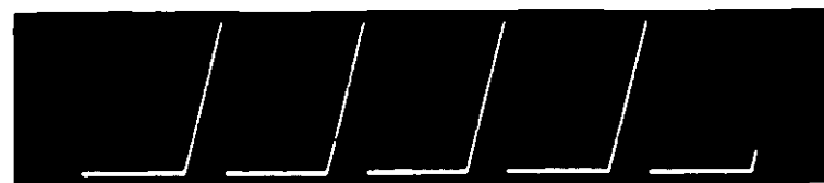
FIG. 6.28(f) (i). EFFECT ON TIMEBASE WAVEFORM ON INCREASING THE SWEEP SPEED SETTING WITH CONSTANT FREQUENCY INPUT
