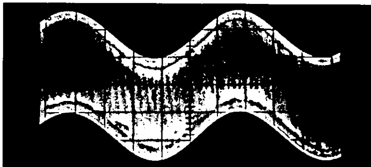
(a) Waveform at low sweep speed showing low frequency superimposed on high frequency. External triggering
